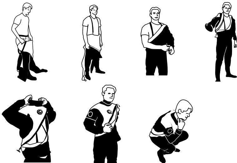
FIG-7 STEPS FOR PUTTING ON YOUR DRYSUIT
